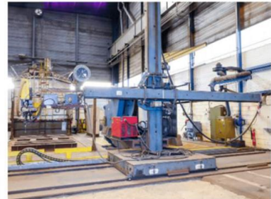
SAF & Boom for SAW welding
