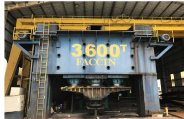
Pressing Machine (Capacity of 3,600Mt)
