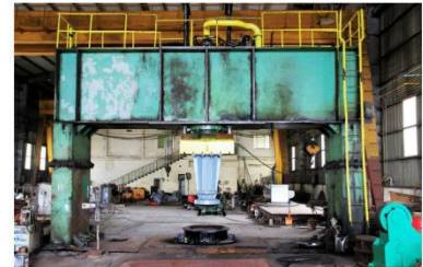
Pressing Machine (Capacity of 1,500Mt)
