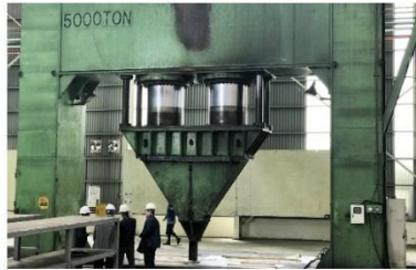
Pressing Machine (Capacity of 5,000Mt)
