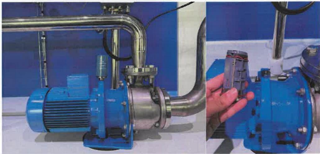
圖 11 AMS Wireless Vibration Monitor
