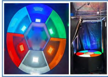
Experimental system for spectral selection preference of eel
