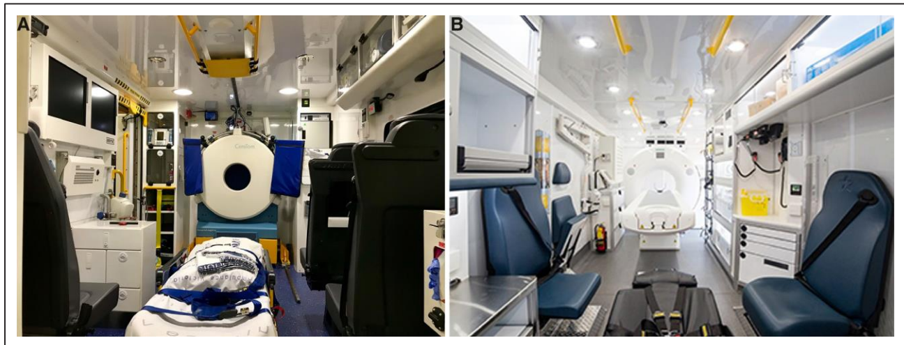
Figure 2. Interior pictures of regular-sized and large mobile stroke units displaying their essential components. Images were provided by PRESTO (Prehospital Stroke Treatment Organization) members from The Royal Melbourne Hospital (A) and the University of Tennessee Health Sciences Center (B).
