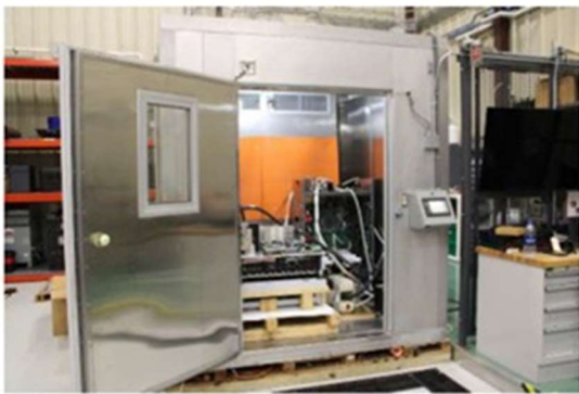
Representative Unit: Thermal Testing While Operating Converter / Cooling System / Vacuum Protection / Electronics
