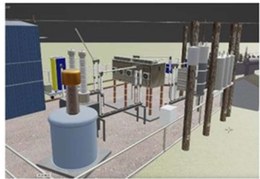
Full Scale: HV Energized – Full Injection Current – Impulse Outdoor Environment with Artificial Wetting
