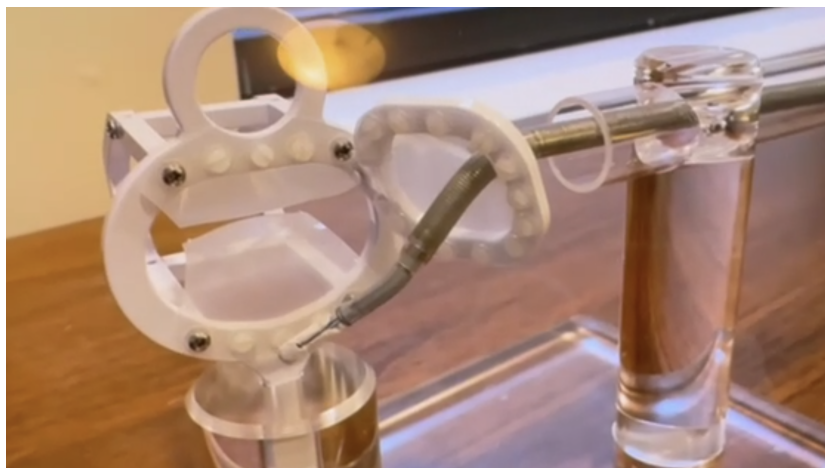
Figure 2.24: TEER system 有許多可動關節與構造，圖片以 MitraClip 為例，顯示 steerable guide catheter (SGC), catheter delivery system (CDS), clip and orientation 之間的關係。
