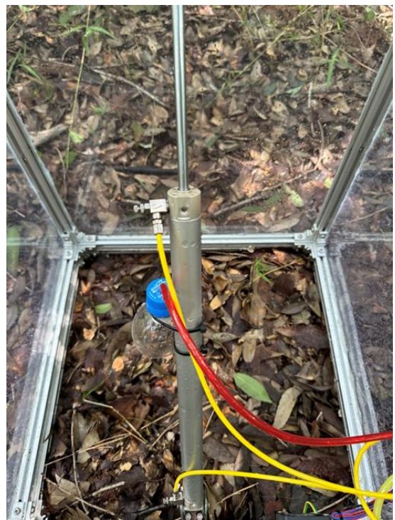
溫室氣體 Automated Chamber System 氣室氣壓缸
