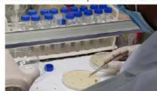
AST profiling by disk diffusion method on fish bacteria samples in WF-KU lab
