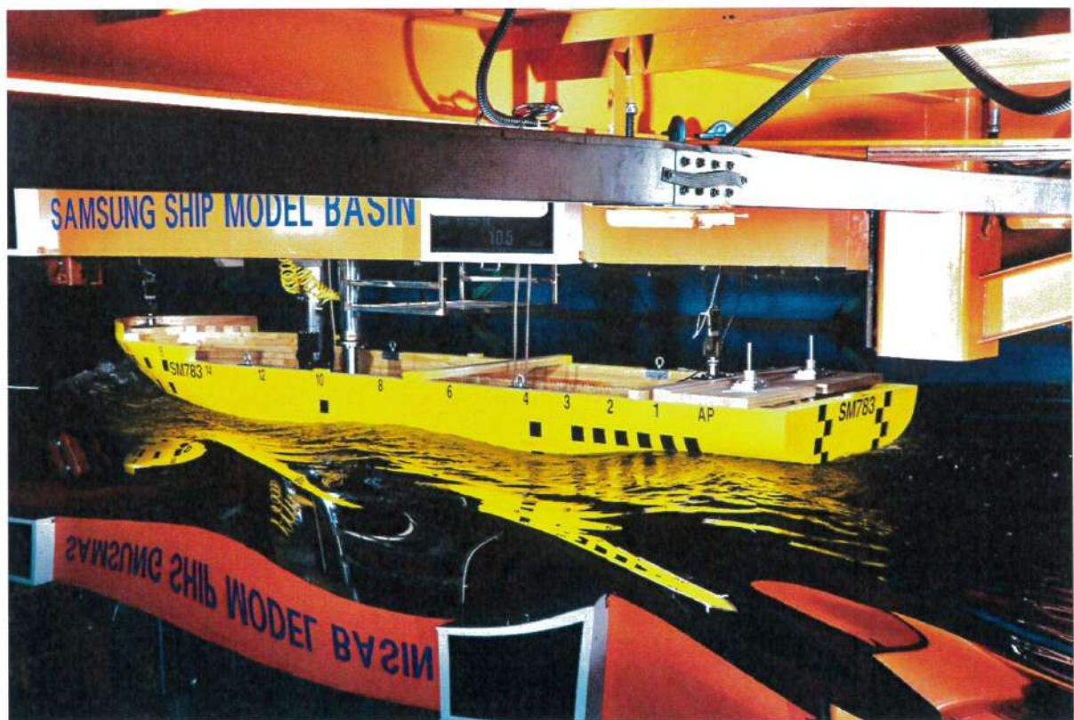
Photo 5 Wave Profiles of Running Model Ship (Design, 10.5 knots)
