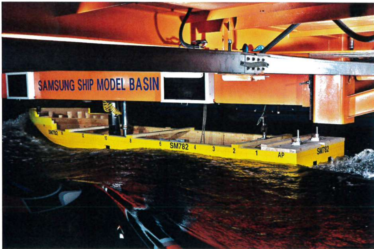
Photo 14 Wave Profiles of Running Model Ship (Scantling, 13.0 knots)
