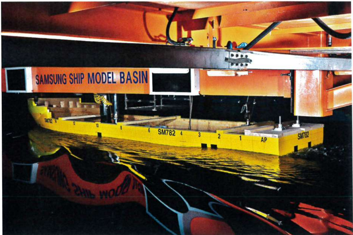
Photo 3 Wave Profiles of Running Model Ship (Design, 7.5 knots)
