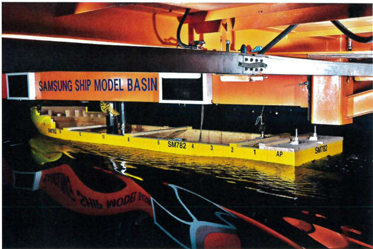
Photo 10 Wave Profiles of Running Model Ship (Scantling, 7.5 knots)
