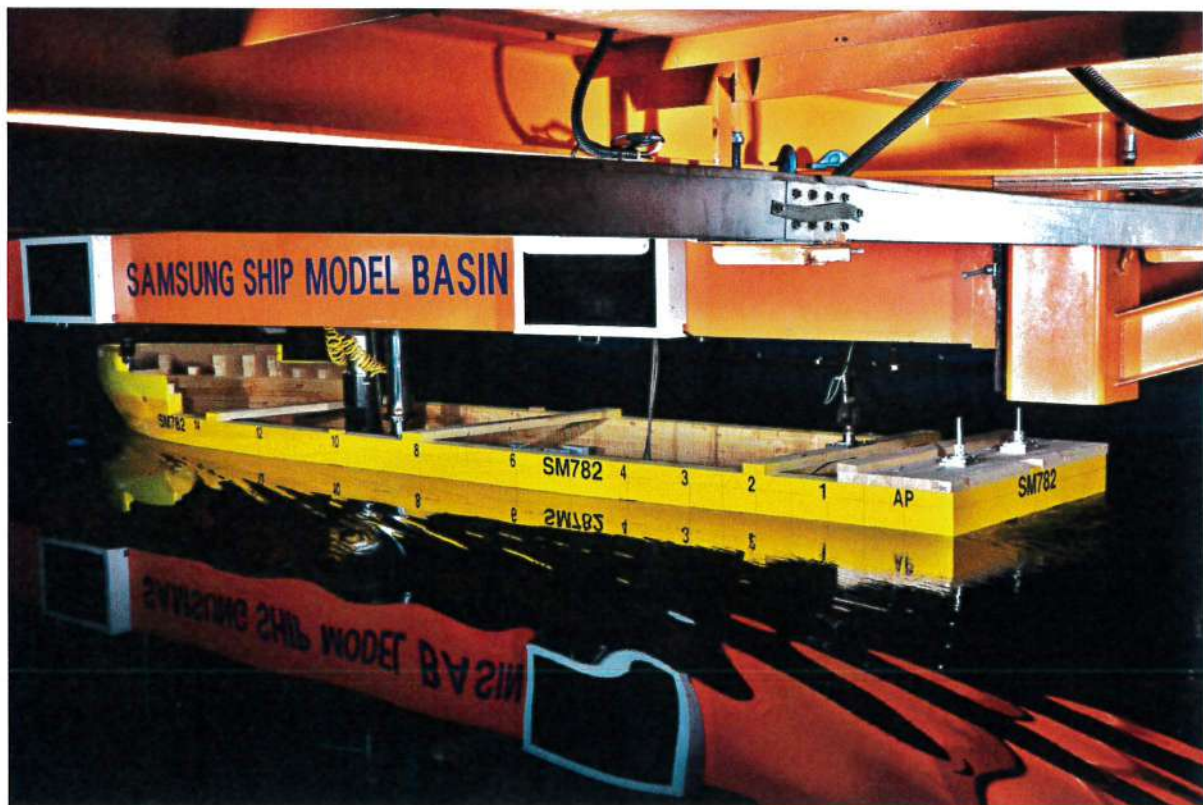
Photo 8 Wave Profiles of Running Model Ship (Scantling, 4.5 knots)
