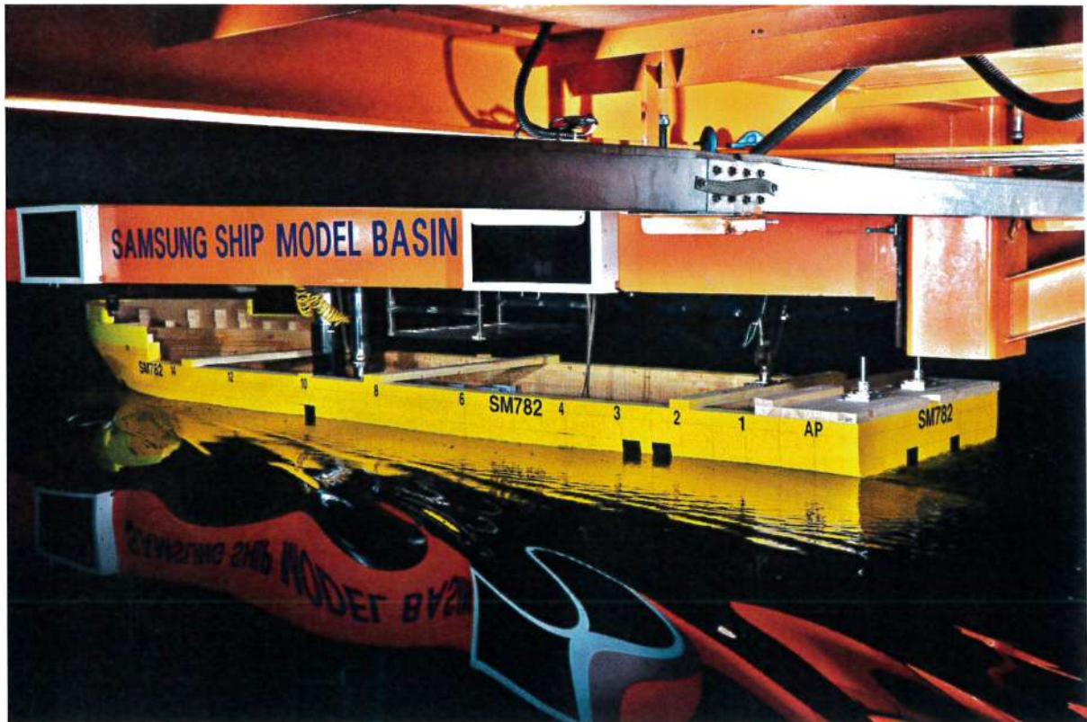
Photo 2 Wave Profiles of Running Model Ship (Design, 6.0 knots)
