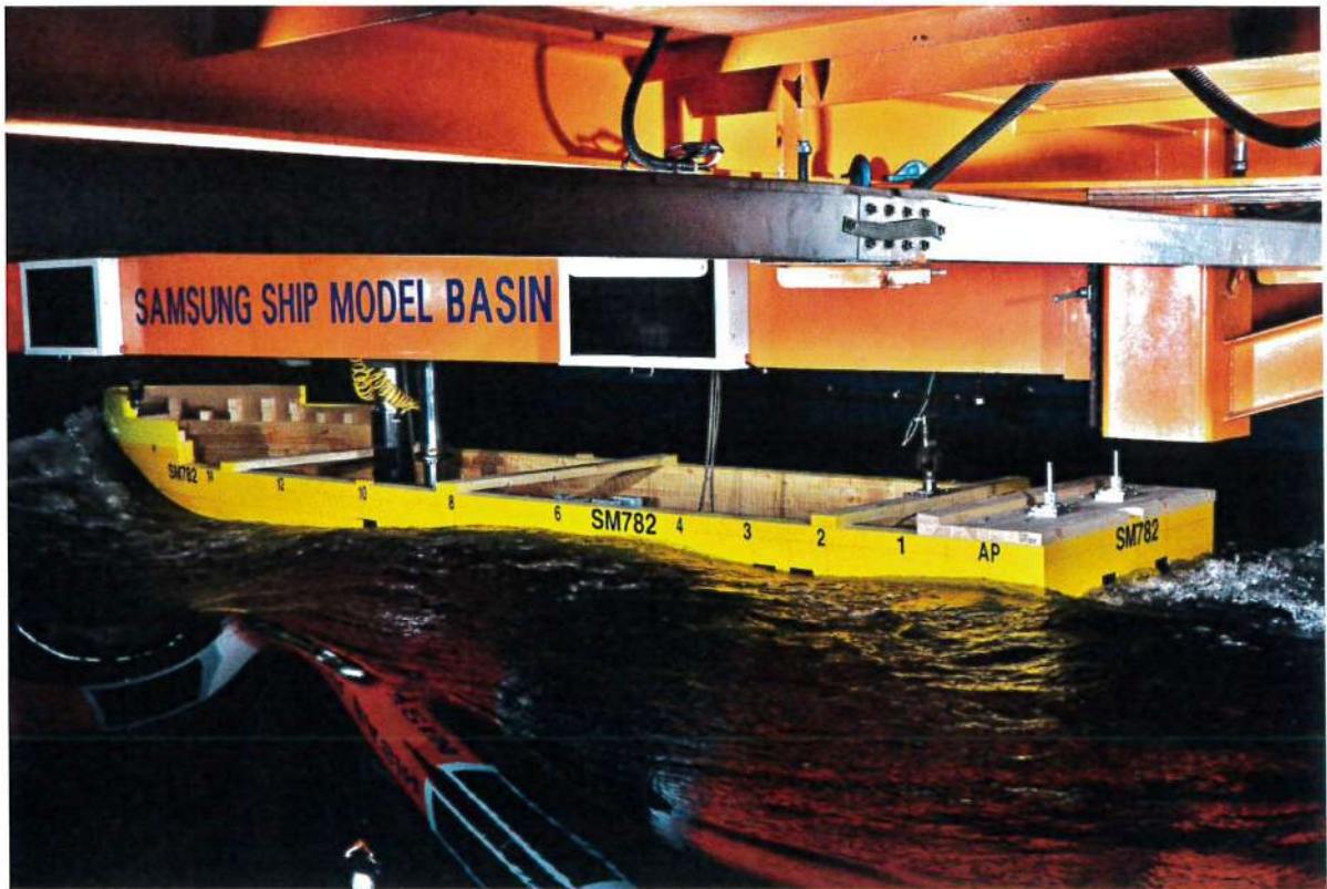
Photo 13 Wave Profiles of Running Model Ship (Scantling, 12.0 knots)
