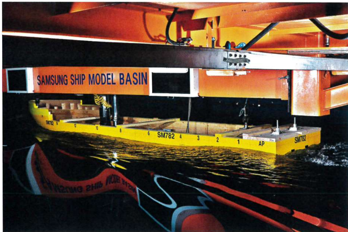
Photo 11 Wave Profiles of Running Model Ship (Scantling, 9.0 knots)
