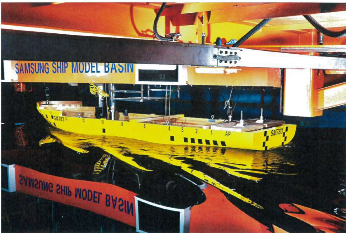
Photo 4 Wave Profiles of Running Model Ship (Design, 9.0 knots)
