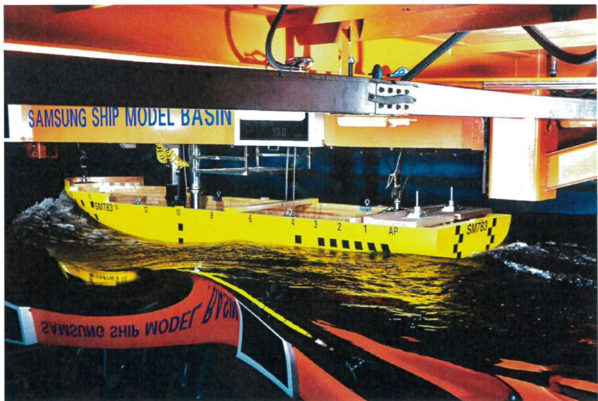
Photo 7 Wave Profiles of Running Model Ship (Design, 13.0 knots)
