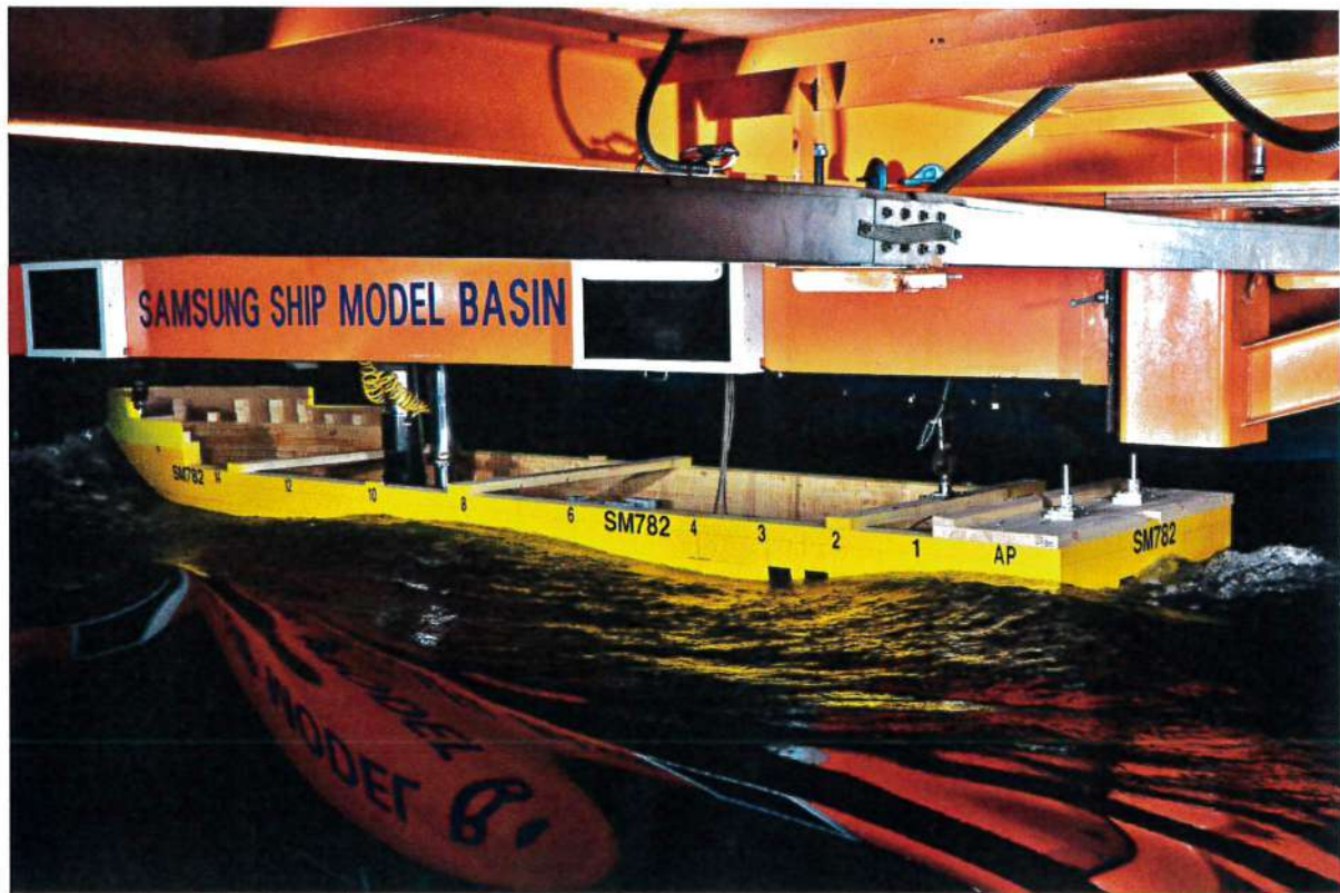
Photo 12 Wave Profiles of Running Model Ship (Scantling, 10.5 knots)
