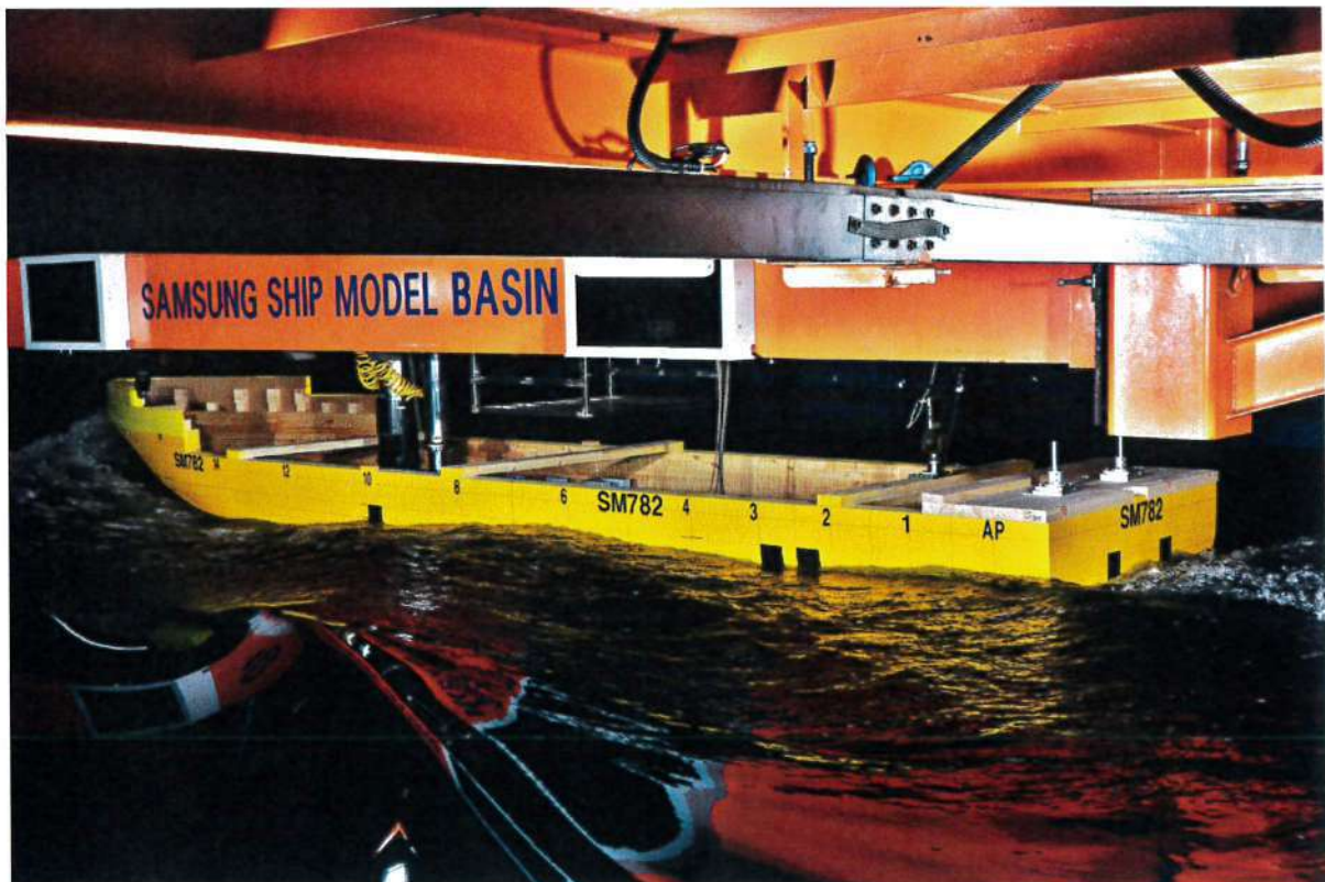
Photo 6 Wave Profiles of Running Model Ship (Design, 12.0 knots)
