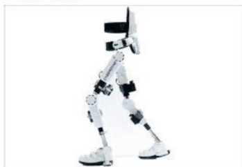
The "HAL® nursing hip type developed by CYBERDYNE" reads bioelectrical potentials and assists with hip movement.
