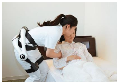
The "HAL® nursing hip type developed by CYBERDYNE" reads bioelectrical potentials and assists with hip movement.
