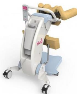
The "HAL® nursing hip type developed by CYBERDYNE" reads bioelectrical potentials and assists with hip movement.
