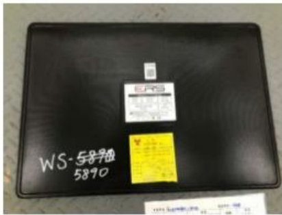
Co-57 source(Nuclear Medicine Gamma Camera Calibration)
