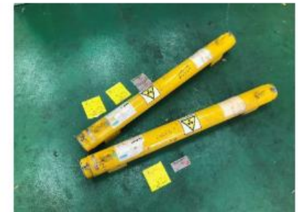
Co-60 source (Density measurement)
