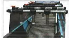
washing and drying at a time by water pressure and air pressure
