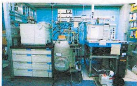
Nano EA (elemental analyzer) / IRMS (isotopic mass spectrometer) capable of measuring the smallest amounts of trace sample isotopes by this type of device worldwide
