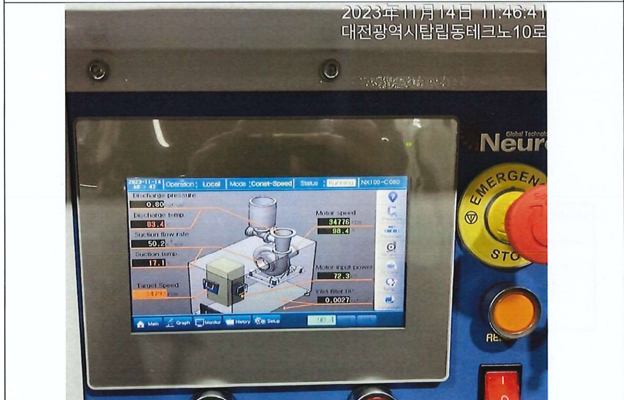
運轉測試額定風壓 = 0.8 \text{ kgf/cm}^2 符合規定 (註: 1000 \text{ mmaq} = 0.1 \text{ kgf/cm}^2 , 8000 \text{ mmaq} = 0.8 \text{ kgf/cm}^2 )
