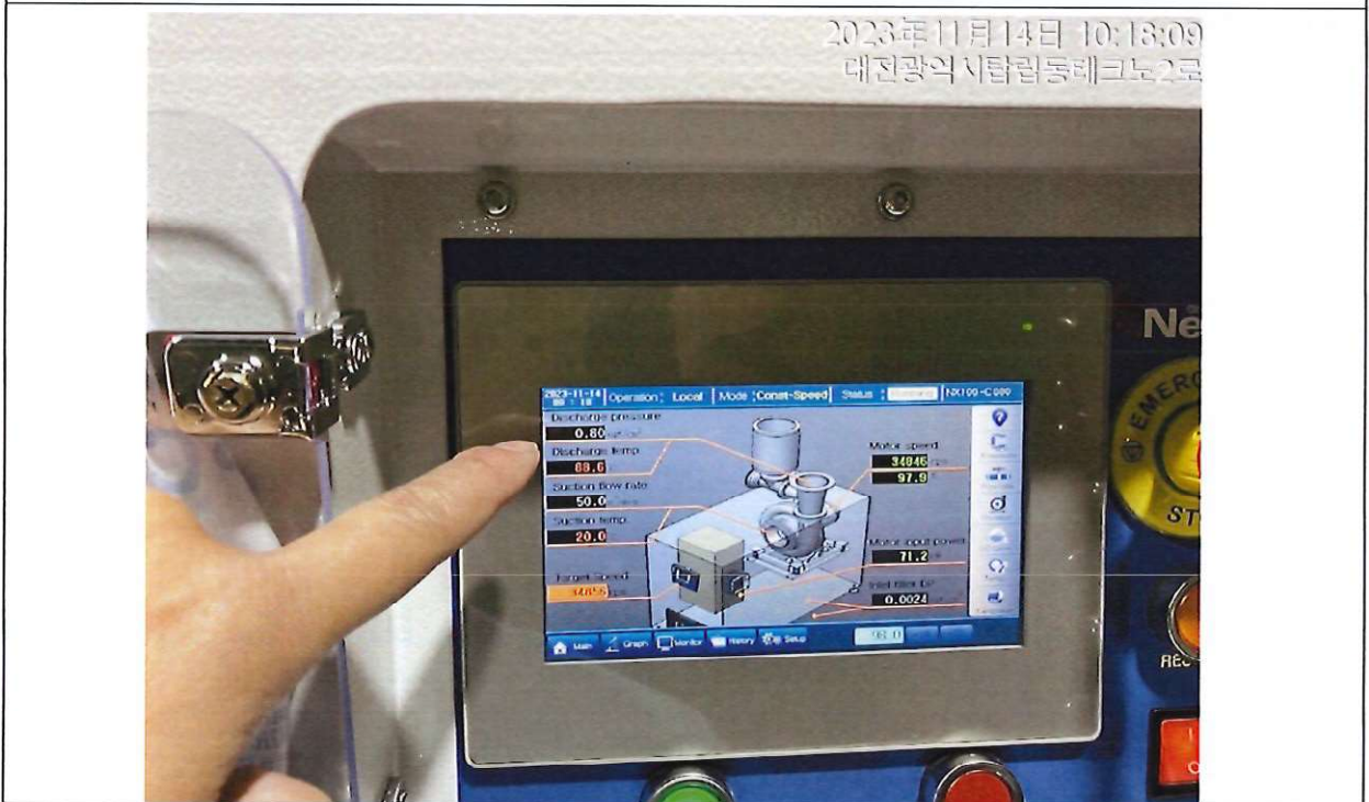
運轉測試額定風壓 = 0.8 \text{ kgf/cm}^2 符合規定 (註: 1000 \text{ mmaq} = 0.1 \text{ kgf/cm}^2 , 8000 \text{ mmaq} = 0.8 \text{ kgf/cm}^2 )
