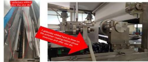
Line Modification to Scale-up of SANIPS\* process
