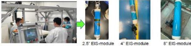
**Customized** spiral wound module fabrication to embed smart sensor allowing in-situ and real-time fouling monitoring of the reverse osmosis (RO) process.
