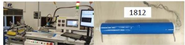
**Customized** spiral wound module fabrication replacing the spacers with electrodes in an electrochemical membrane system to achieve in-situ low-energy and chemical-free regulation of solution pH.
