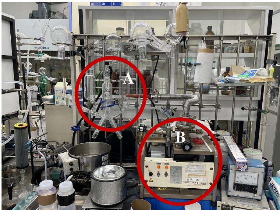
圖9、溶劑輔助風味蒸發萃取裝置(Solvent assisted flavor evaporation, SAFE)
