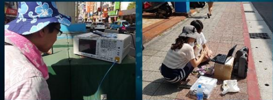
Measure and record RF work band signal strength and background noise.
