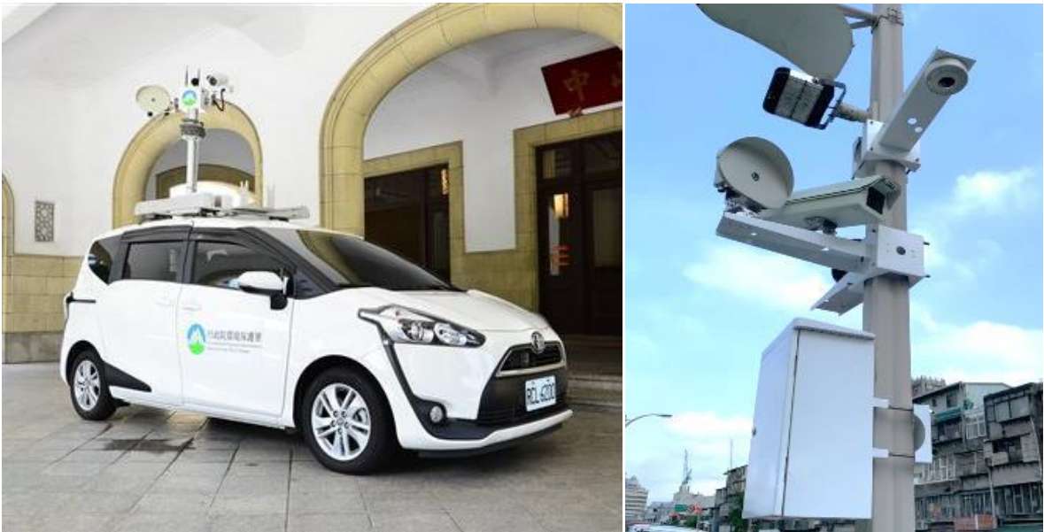
Figure 3 The initial prototype of acoustic camera system ( Left: vehicle type / Right: fixed type )
