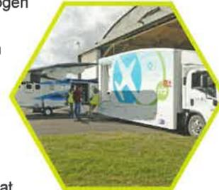
The refuelling solution takes hydrogen gas and compresses it up to 450 bar. It is capable of dispensing up to 20 kg hydrogen at 350 bar per operation.
