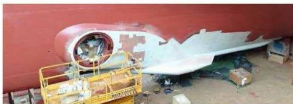
No gondola => same draft kept A fairing under the keel
