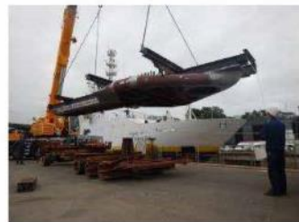
No gondola => same draft kept A fairing under the keel
