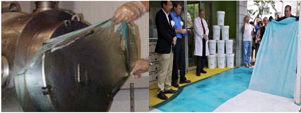
圖 20、可剝離高分子聚合物除污操作示範圖(Source: Ofra Paz Tal, Decontamination Processes and Techniques: Polymeric Gels)
