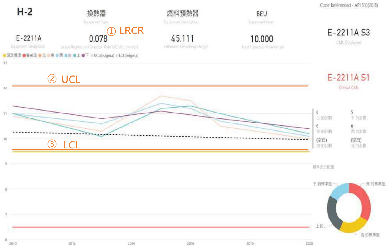
Figure 2: Control Chart with Linear Regression Corrosion Rate and Other Information
