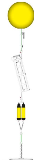
Mooring diagram. From top to bottom, mooring includes a float, AZFP instrument, tandem releases, and anchor.
