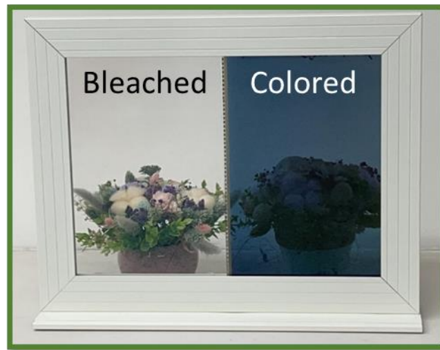
Fig. 5. Performance of Energy-Saving Window (area: about 400 \times 300 \text{ mm}^2 )
