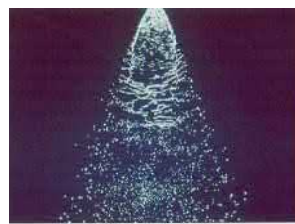
Spray pattern produced by a pressurised nozzle, showing the large range of particle sizes produced
