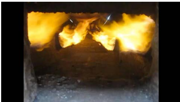
Syngas is burnt to produce heat for drying waste before transferring them into the gasification reactors.
