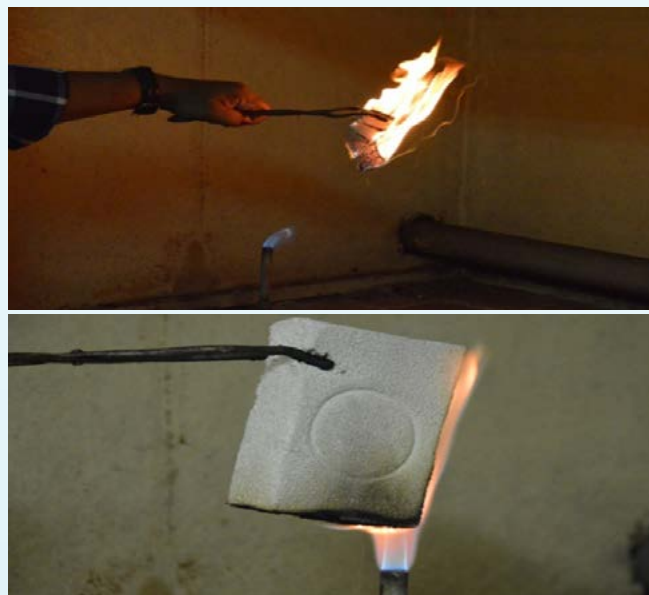
Fig. 2 Images of commercial polyurethane foams set to fire. (Left)-foam without CASPOL impregnation burned completely in fire within a few seconds whereas CASPOL impregnated foam (right) remained intact even in fire.
