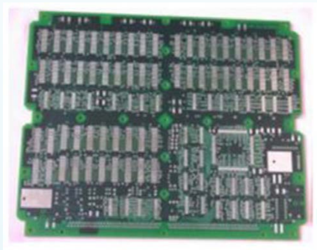
Fine Line SSR Multiplayer PCB Replaced 6 Normal MLBs
