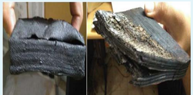
Coated v/s bare wood specimen at 400°C
