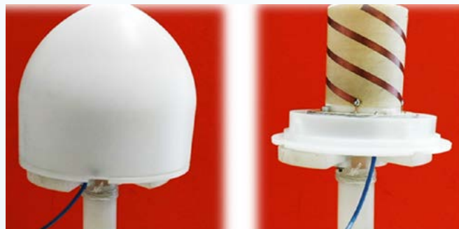
Tx Antenna for Pole
