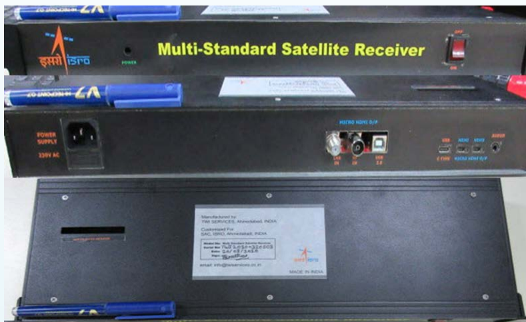
Integrated module, size:1U (can be further decreased by vertical PCBs stacking)
