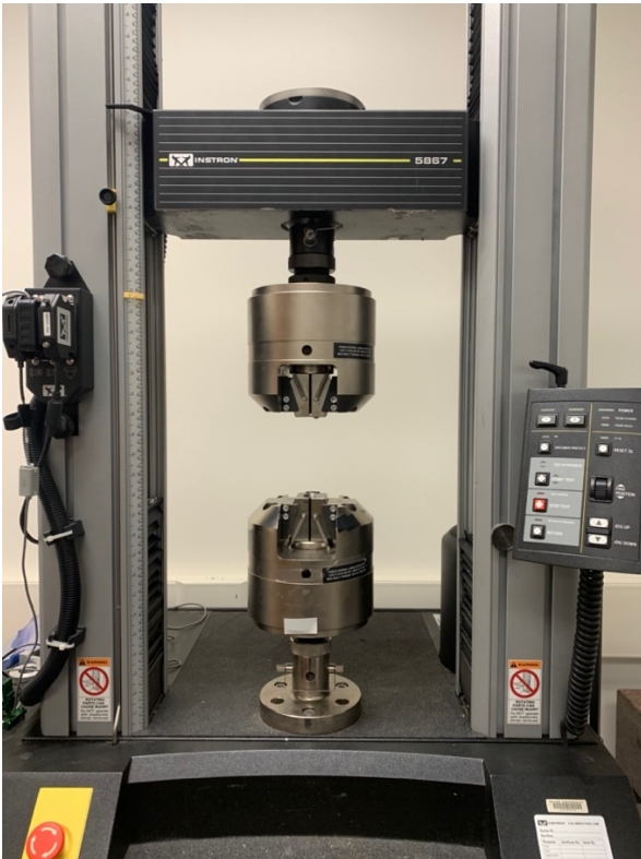
Figure 12 INSTRON 5867 compression/tensile machine
