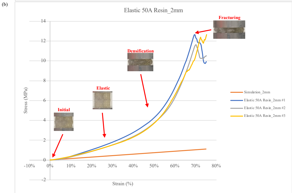
Figure 43 Cross Cube + BCC + Octahedron (Elastic 50A Resin) - Compression Test and Simulation Results: (a) 1mm truss diameter, (b) 2mm truss diameter
