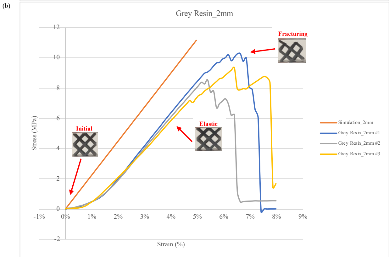
Figure 22 BCC (Grey Resin) - Compression Test and Simulation Result: (a) 1mm truss diameter, (b) 2mm truss diameter
