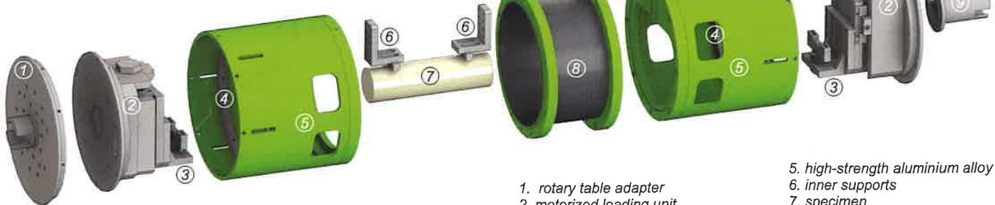
Configuration of the 4PB loading device
