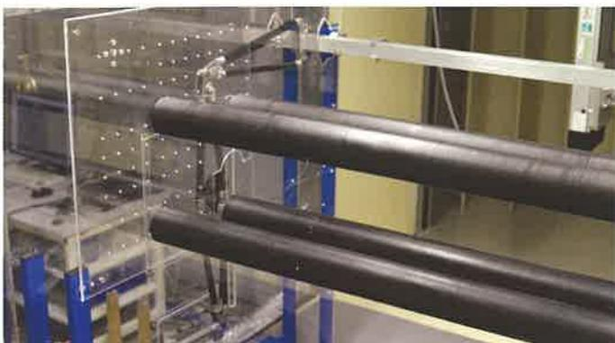
Aeroelastic model of four hangers placed in the wind tunnel
