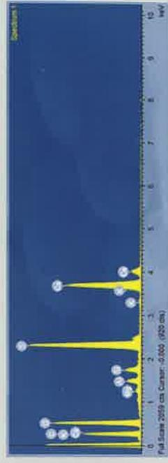
EDS spectrum of gypsum crystal at the surface of aggregate
