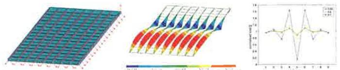
Fig. 2 a) Model of rafter set created by ANSYS software, b) distribution of bending moment, c) influence of all-wooden joint application (position no. 5) on strain distribution in the other structural elements after being fully loaded (values of model bending stiffness  $k_{model}$  – missing element  $k_{model} = 0,05$ , joint positioned in the third of element  $k_{model} = 0,5$ , joint close to element end  $k_{model} = 0,7$ ).
