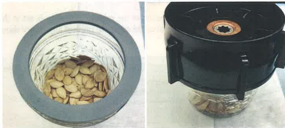
Figure 3. Assembly of base, blade, rubber seal and jar.
