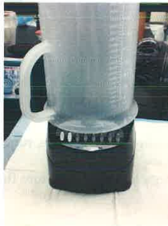
Figure 5. The jar-blender bottom assembly is covered by a 3L plastic beaker as a precautionary measure if glass jar breaks during grinding. Alternatively, a large plastic yogurt container may also be used for this purpose.
