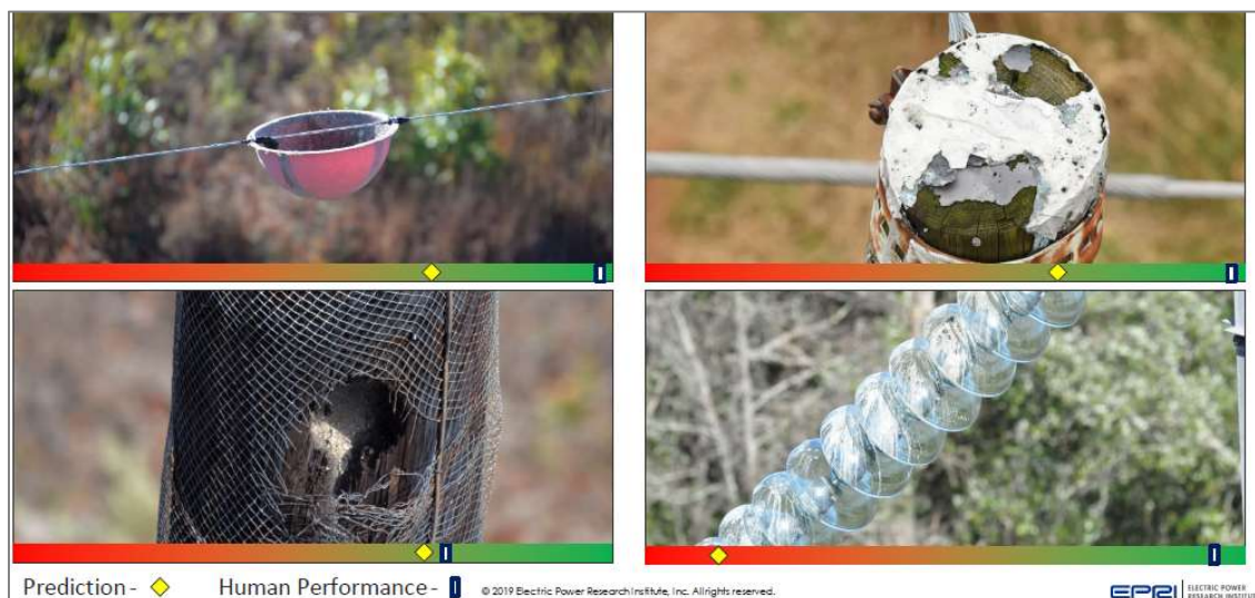
圖31 AI影像辨識(Pattern Recognition)故障圖案
