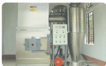
Medical solid waste incinerator VHI-18B (Patent and trademark awarded product)
