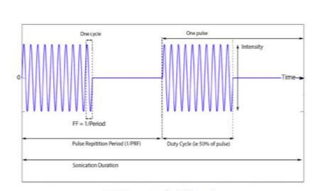
Fig. 1. Key parameters of pulsed ultrasound.
