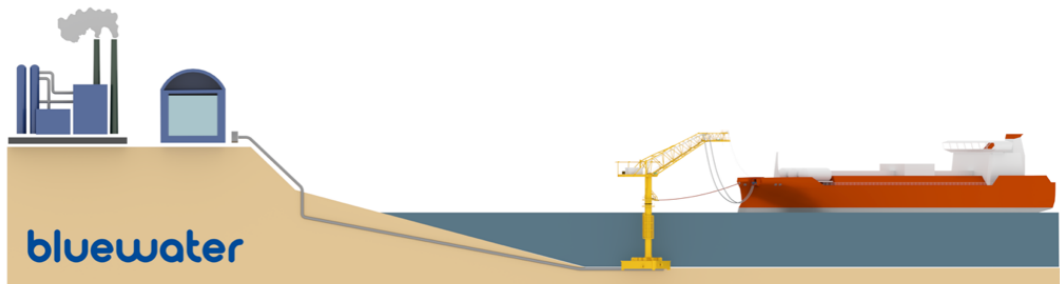
(Yoke mooring system 應用示意)
