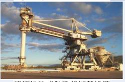
連續性乾式散雜貨卸載設備 (Continuous ship unloader)
