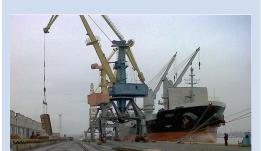
通用貨物卸載吊車,可換吊車頭下載 貨櫃(Containerized ship loading)(Dry bulk)
