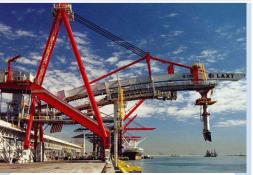
高效能的乾式雜貨卸載設備(Dry cargo equipment, high capacity)(9000 tones/hr)
