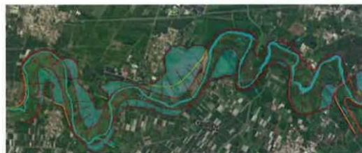
Blue: river; Red (dashed line): original dyke; Red (solid line): new dyke
