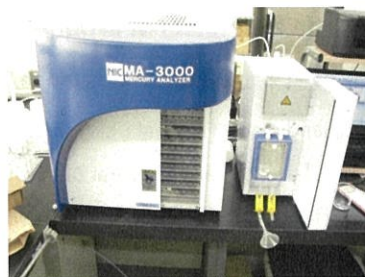
MA3000 (left side) : Atomic absorption spectrometer RH-MA3 (right side) : Thermal desorption device (option)
