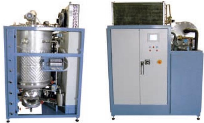
Can be used for process water that has a strong tendency to become caked during evaporation. A continuously rotating stainless steel brush prevents the formation of deposits that would reduce the heat transfer capacity.
