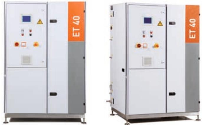
Mechanical exhaust compression is used for reuse of the energy contained in the vapour. The ducted-overflow condensing heat exchanger and the consistent use of the heat from the distillate enable the low energy consumption of 40 watts per litre. The regulation of the compression and an integrated distillate after-treatment by a coalescing device achieve best distillate qualities.
