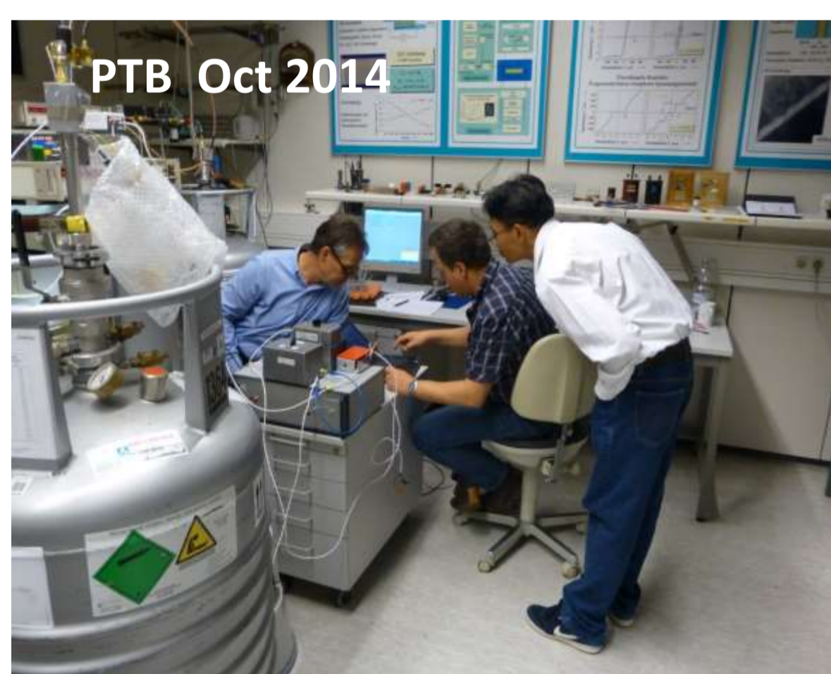
BIPM.EM-K10.b: comparison of Josephson voltage standards at 10 V
