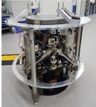
A 6DOF micro-vibration measurement/generation test facility (NPL)
