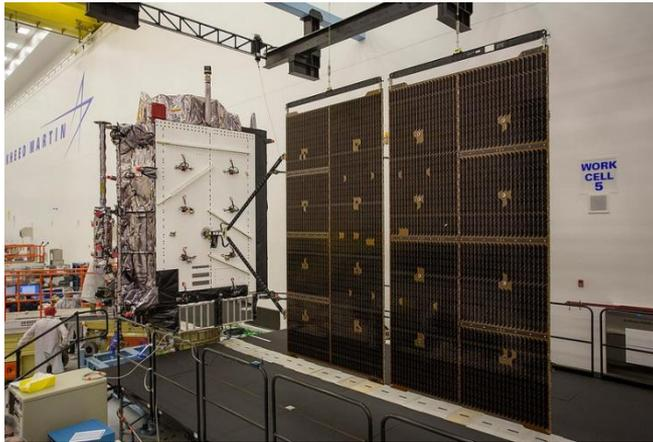
GPS III SV02 Array Deployment Test
