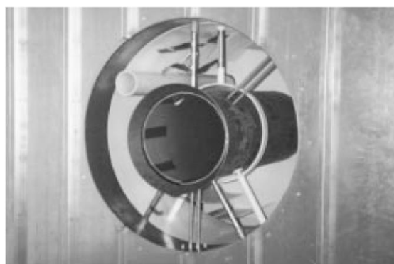
IBAM™ Probe Calibration Testing in AMC's Wind Tunnel Facility
