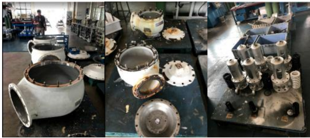
Safety relief valve 工廠拆解保養
