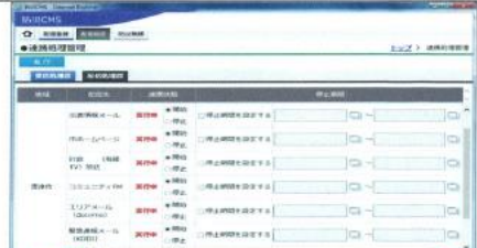
Karatsu City disaster management information interfacing system (Multiple public communication media can be actuated simultaneously from a single terminal)
