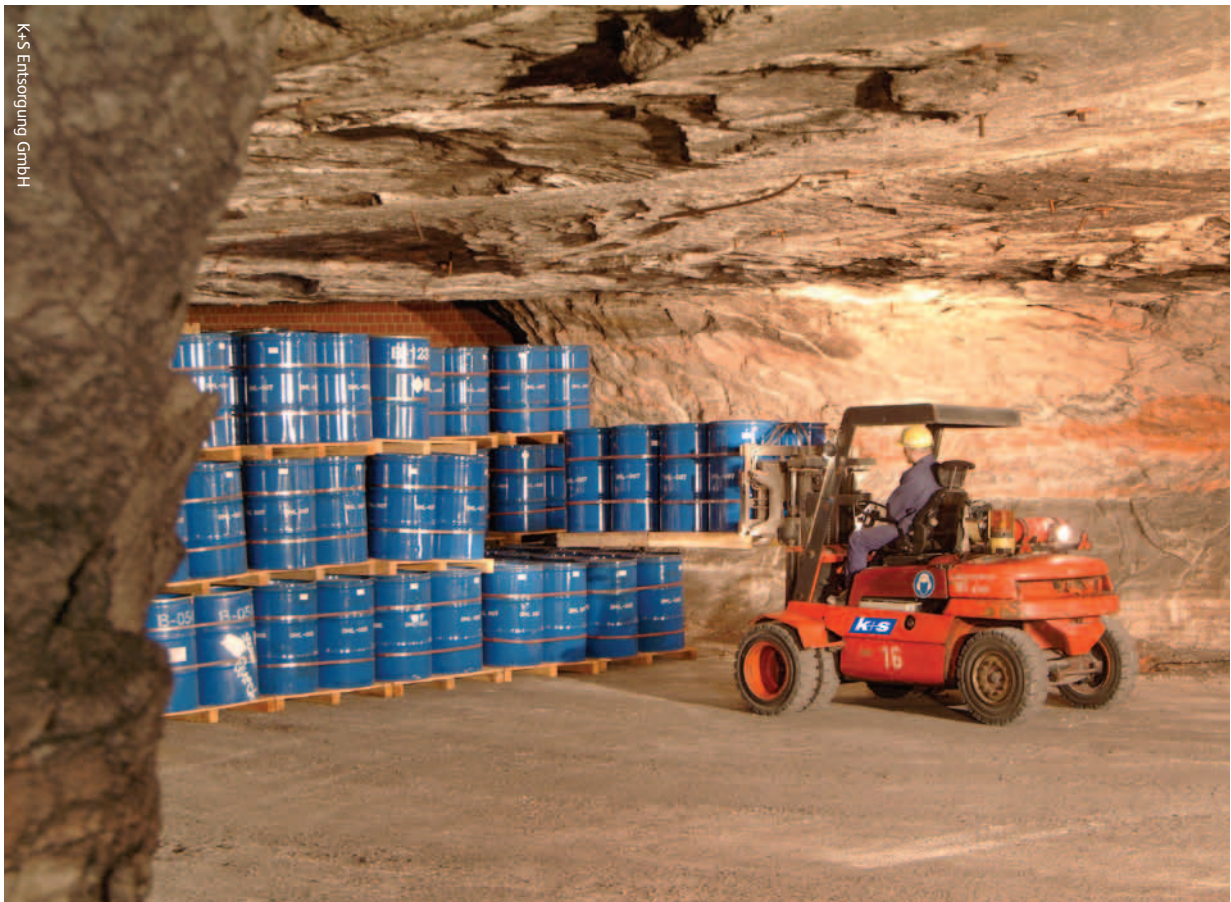
Recovered mercury is being stockpiled at long-term storage sites above- and, as shown here, below ground.
