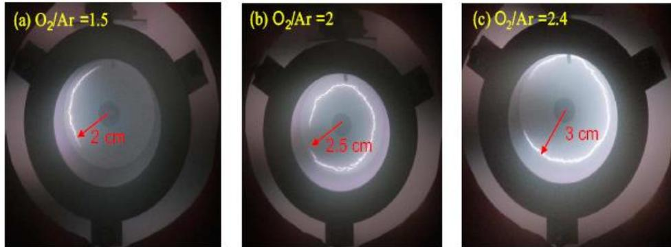
Figure 2 Schematic images of cathodic spot motion under different relative ratio of oxygen and argon
