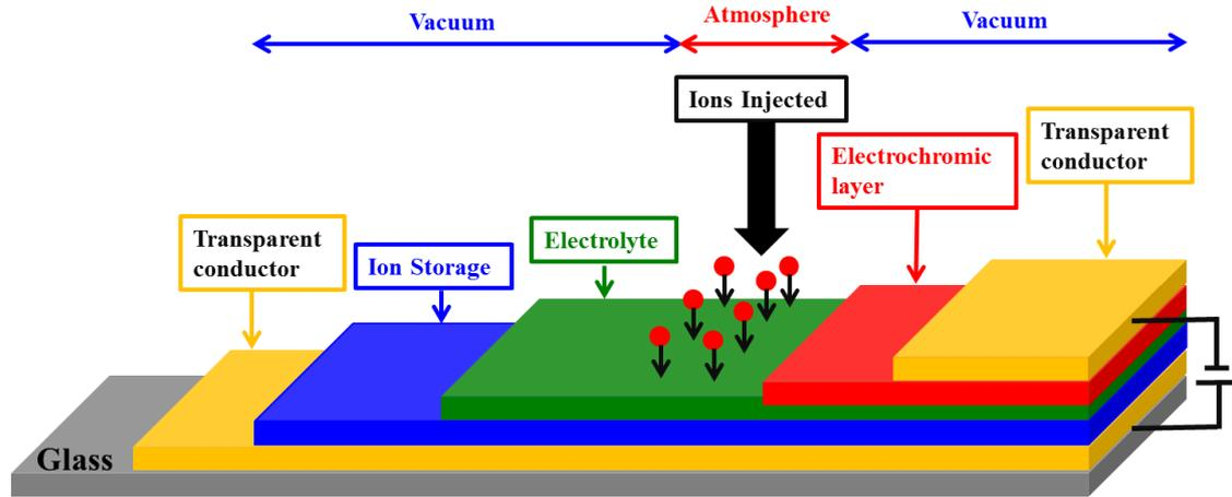
Figure 1. The typical structure of electrochromic device.
