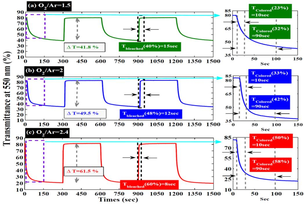
Figure 3 Temporal switching time characteristics between bleached states and colored states for the  $\text{Ta}_2\text{O}_5$  with electrolyte ECD for different relative ratio of oxygen and argon using applied voltages of +3.5 V (bleached state) and -4 V (colored state) while the duration time were fixed at 300 s (@550 nm). Inset Figure 3 (a) - (c), we are shown shortly duration time for 150 s
