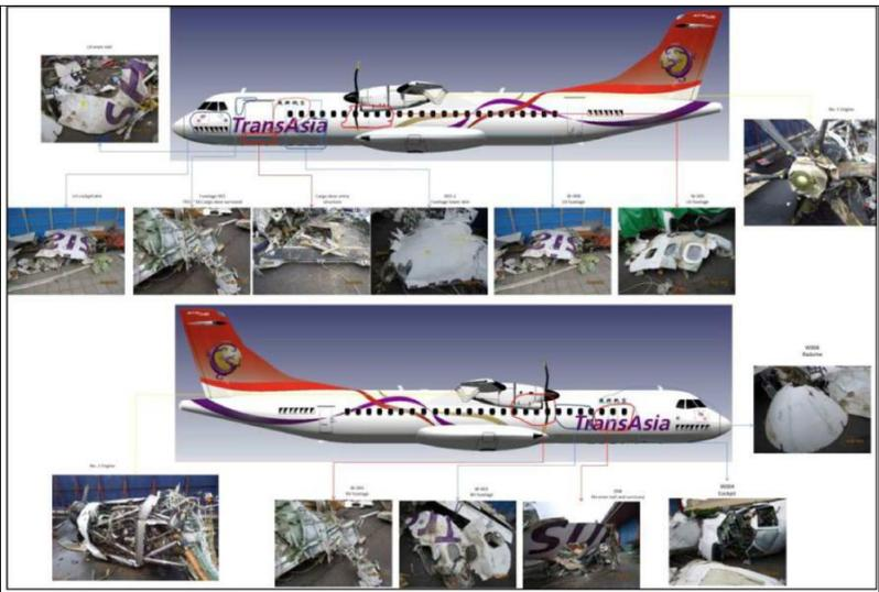
Figure 1.12-3 Recovered aircraft wreckage (2)
