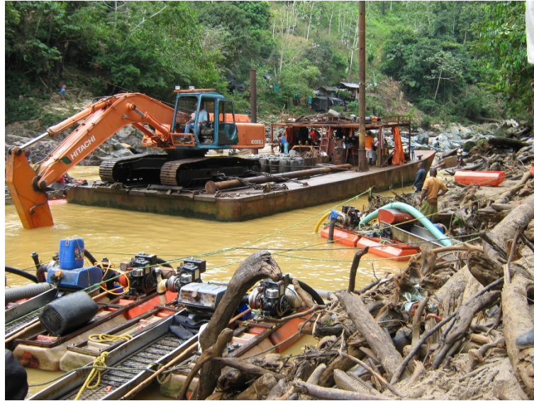
Picture 2. Pontoons and dredges mining alluvial gold
