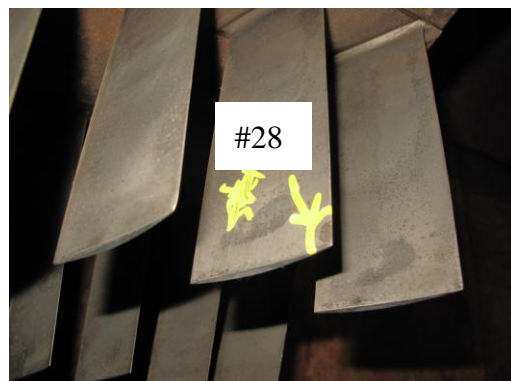
#28 塗層脫落，範圍 (4 \times 6) \text{ mm}^2
