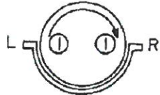
POSITION 1 WITH #1 BOLT HOLE OF COMP ROTOR AT LEFT
